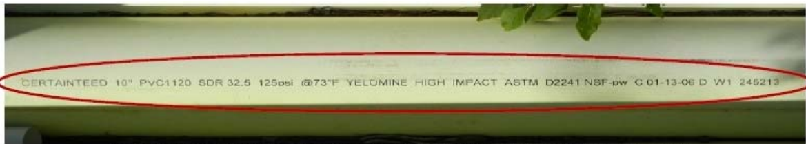
TUBERIA INSTALADA EN LINEA SUBMARINA CHIQUILA-HOLBOX, CERTA-LOK YELOMINE DE 10"Ø
