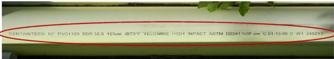
TUBERIA INSTALADA EN LINEA SUBMARINA CHIQUILA-HOLBOX, CERTA-LOK YELOMINE DE 10"Ø
